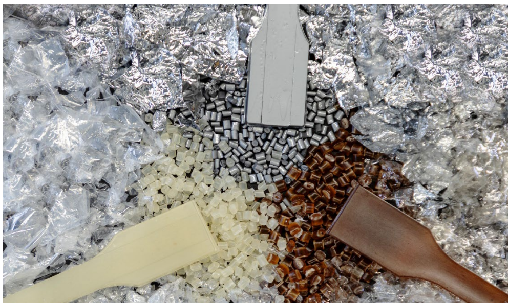
Fig. 05: Recycled granulate from different waste films and produced dog bone samples [Fraunhofer ICT–2023].
